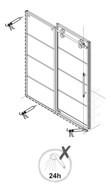
Do not use the shower enclosure for at least 24 hours in order to allow the silicone sealant to cure fully.
