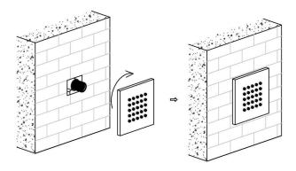
3. Use a hexagonal wrench to rotate clockwise to install the 1/2 threaded joint on the wall side spray joint. (Note: The 1/2 threaded joint has an internal threaded end facing outward).
