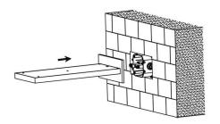
10. Tighten the M6X8 screw by hex tool to secure the showerhead.
