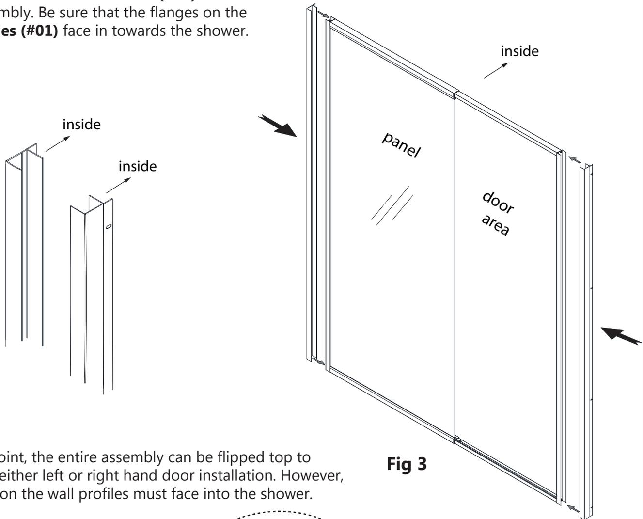
**4.** At this point, the entire assembly can be flipped top to bottom for either left or right hand door installation. However, the flanges on the wall profiles must face into the shower. **(Fig 4)**
