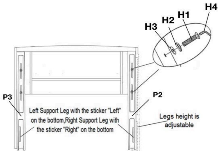
Put the Headboard onto a flat surface. Align the mounting position on Headboard to the mounting position on Left Support Leg(P2). Then, lock the top and the middle mounting positions by Flat washer (H3), Spring washer(H2), bolt(H1), Then tighten the bolts with allen wrench (H4) . Repeat the same steps to install the Right Support Leg(P3). At this point of assembly, DO NOT overfasten the connections. The final height of the Headboard may be adjusted to your own need.
