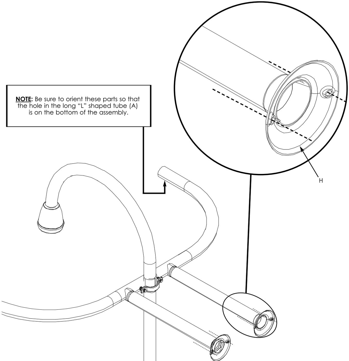
12. Attach the assembly to the wall. **NOTE:** If you screw directly into studs, anchors (T) are not necessary.
