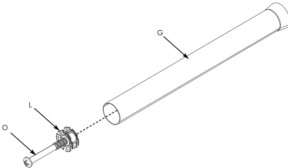
7. Unscrew large screw (O), leaving metal insert (L) inside the tube. Repeat, using other cut flared tube (G).
