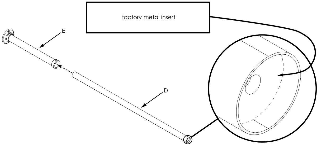
19. Insert 7/8 in. nylon insert (N) into the end of long straight tube (D). Fasten long straight tube (D) to the assembly using a large screw (O).
