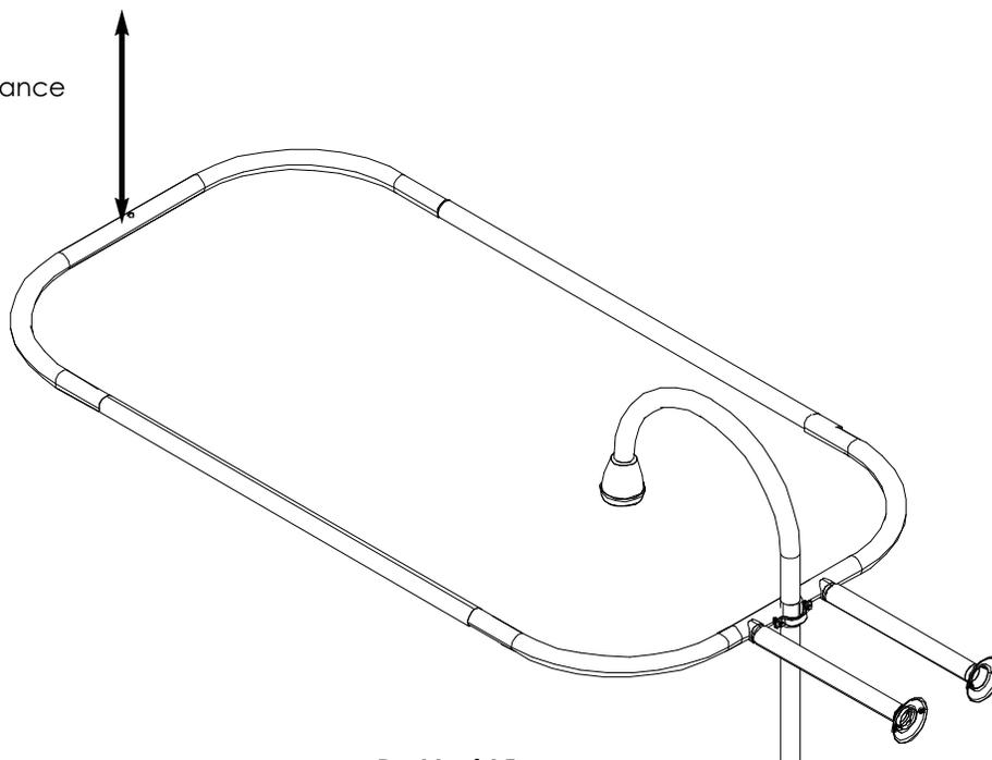
16. Subtract 2 in. from the measurement from step 15. Measuring from the end of the tube **with the factory metal insert**, mark this measurement on long straight tube (D). Using a hacksaw, cut long straight tube (D) at the mark.
