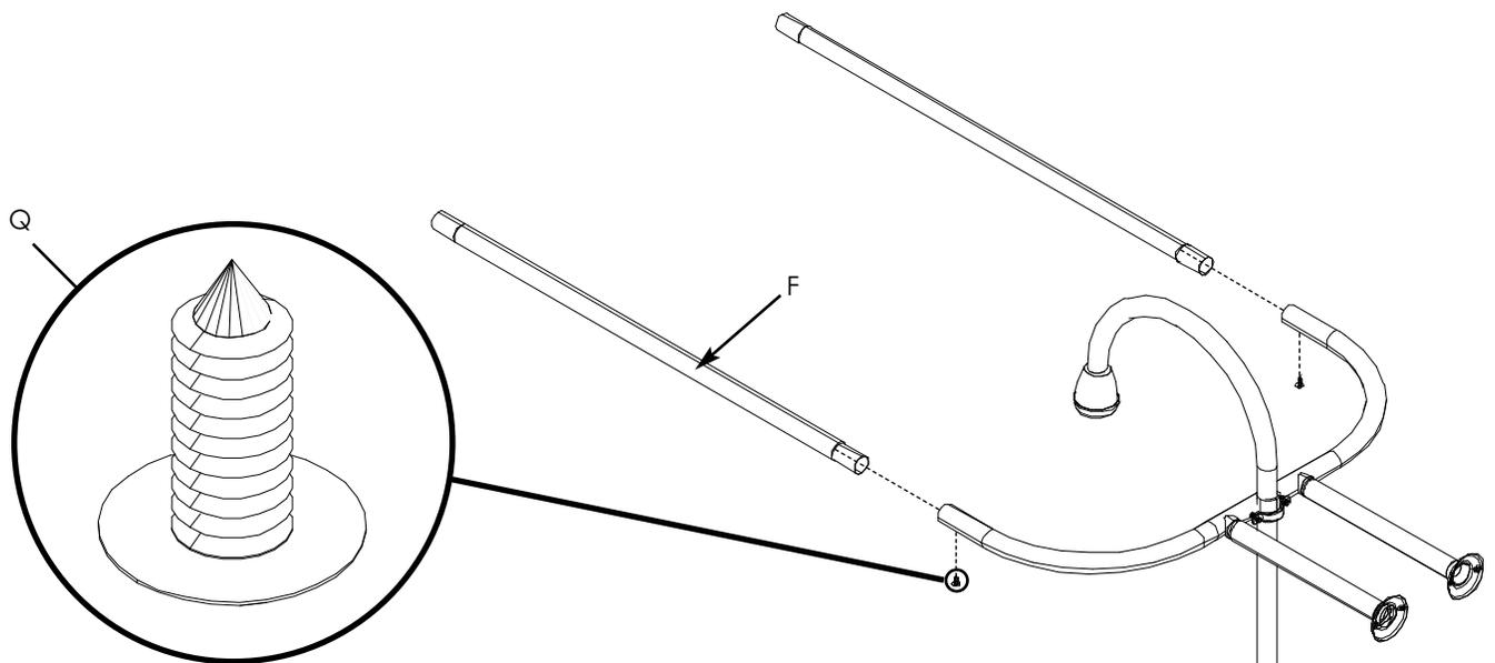
14. Attach U-shaped tube (C) to the assembly using small screws (Q).
