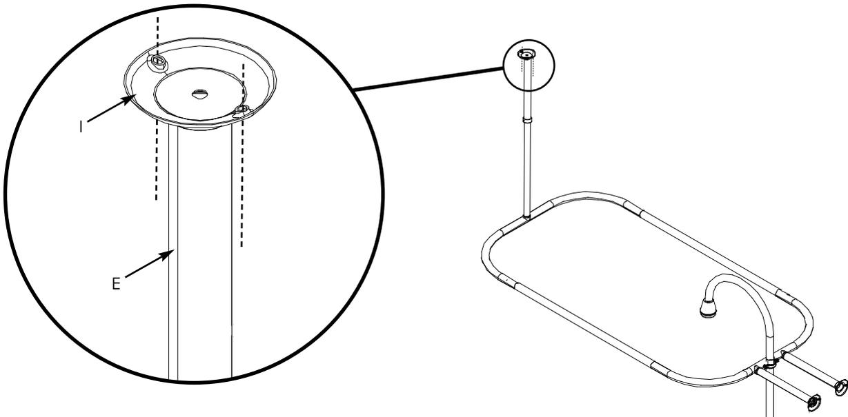
21. Using mounting screws (S), attach closed metal flange (I) to the ceiling, as shown.
