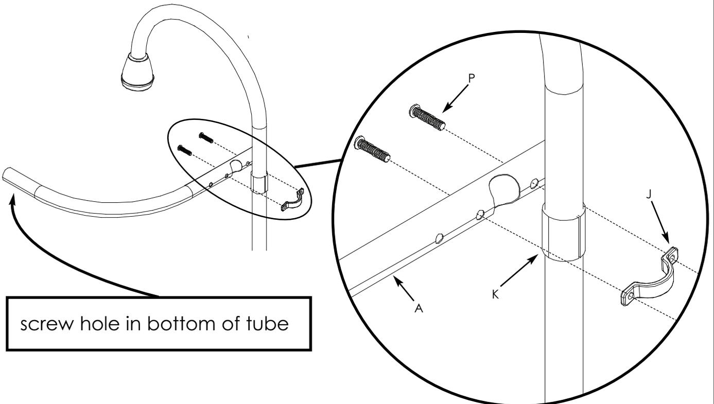
3. Measure distance from long "L" shaped tube (A) to wall.
