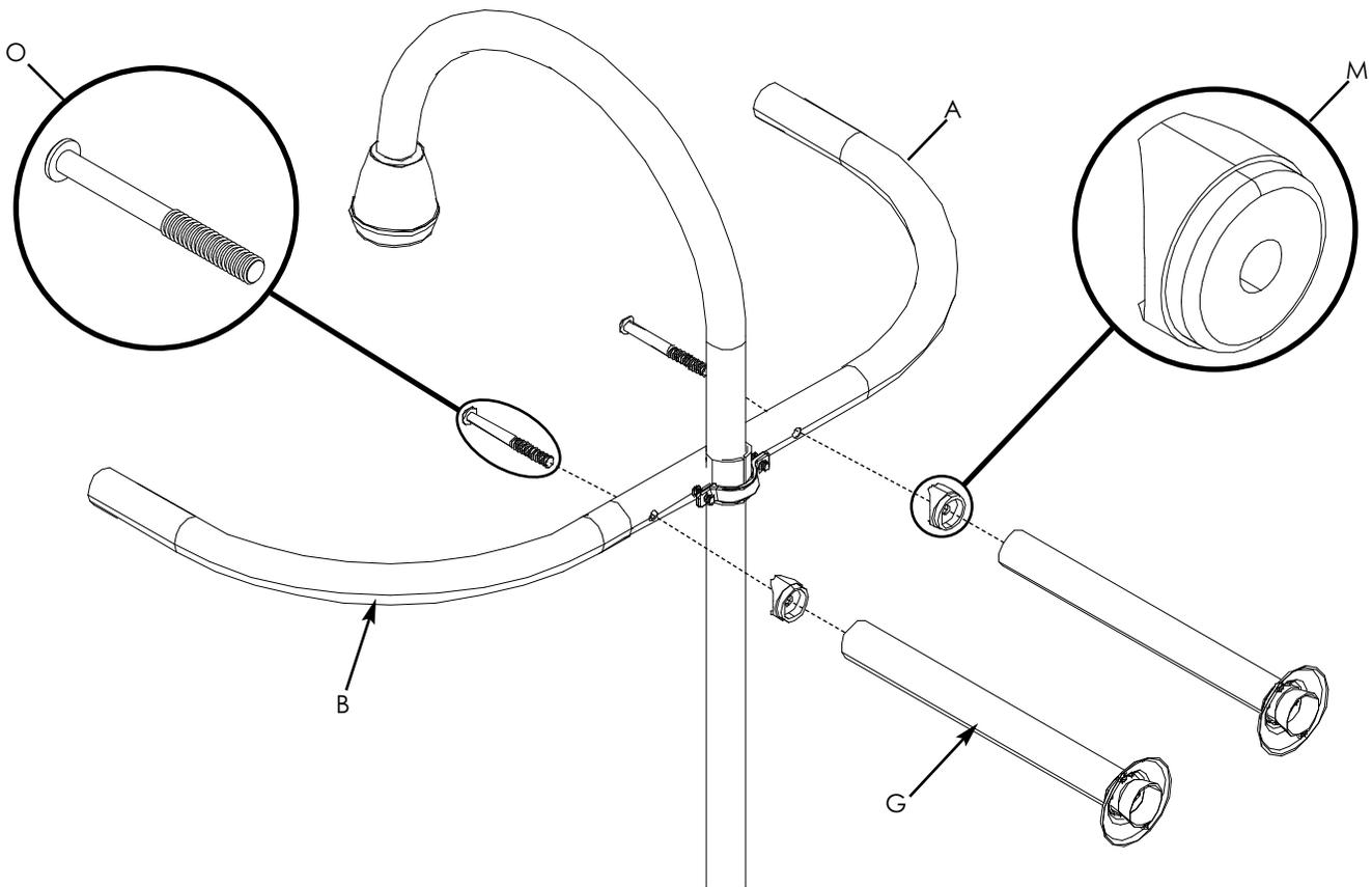
**NOTE:** If nylon inserts (M) can't be inserted inside of flared tubes (G), metal inserts (L) may need to be inserted a little farther into flared tubes (G). (See step 6.)
