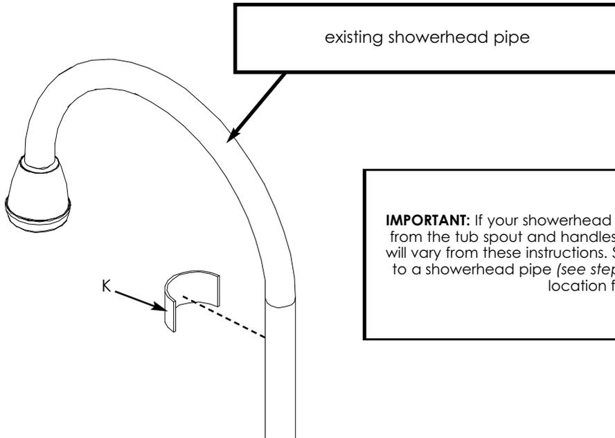
**IMPORTANT:** If your showerhead pipe comes out of the wall instead of up from the tub spout and handles (see photo on page 1), your installation will vary from these instructions. Since the shower rod will not be fastened to a showerhead pipe (see step 2), you will have to determine the best location for the shower rod.
