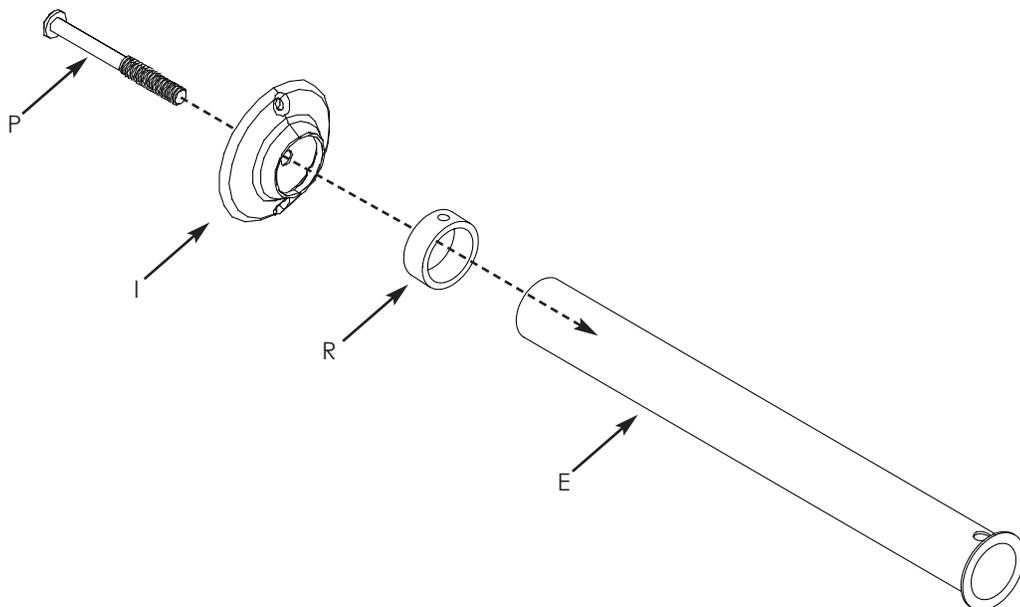
18. Slide the long straight tube (D) that you previously cut into short tube with hole (E), as shown.
