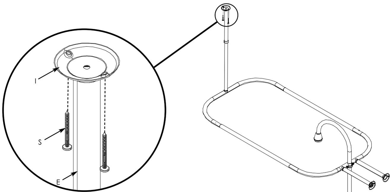
22. **NOTE:** Make sure the rod assembly is level.
