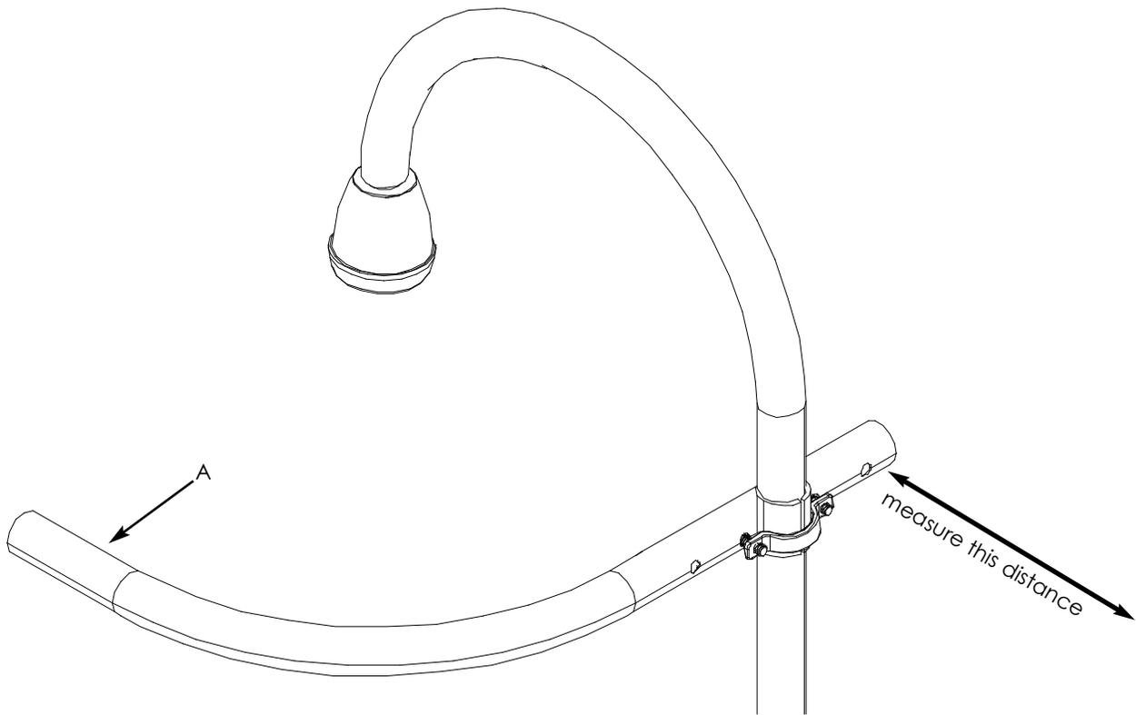
4. Subtract 1/8 in. from the measurement in step 3. Measuring from the **flared-end** of the tube, mark this measurement on flared tubes (G). Using a hacksaw, cut flared tubes (G) at the mark.
