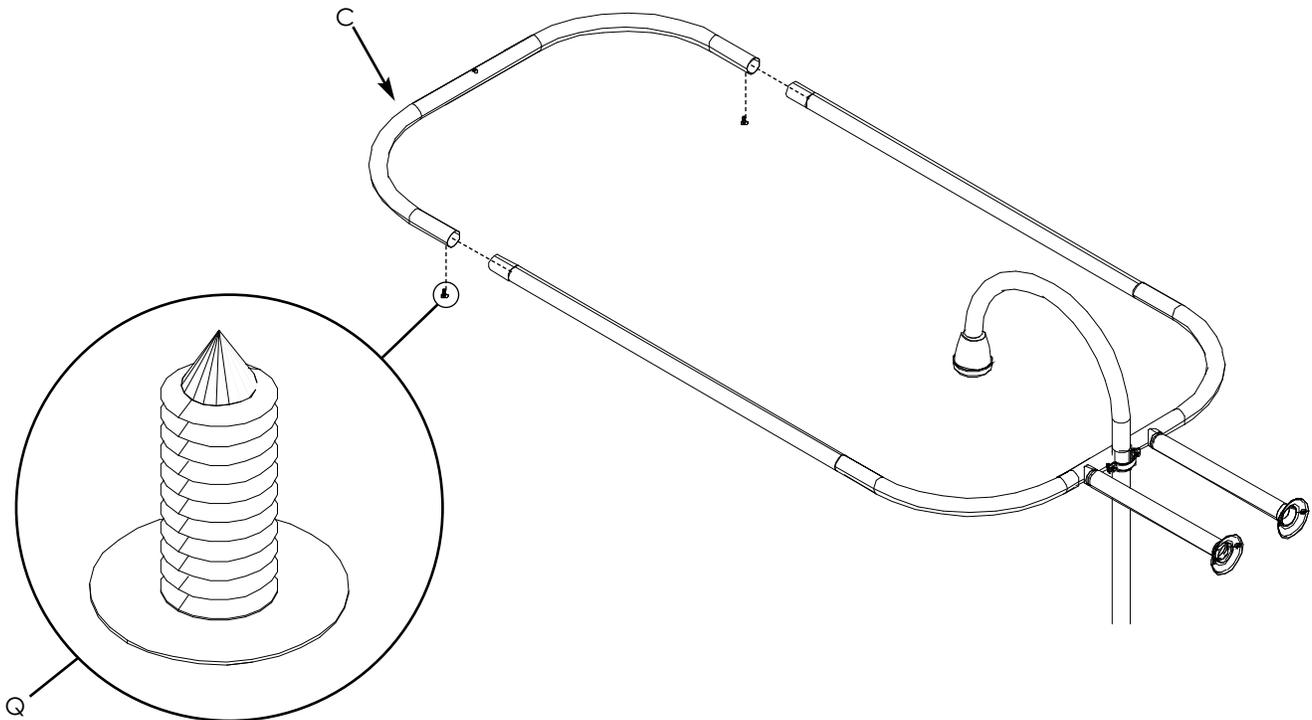
15. Keeping assembly level, measure from the top of assembly to ceiling.
