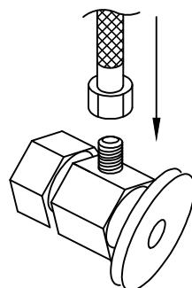
4. Connect female end of flexible hoses to the cold and hot water supply.
