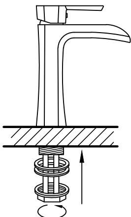
3. Place new faucet in the position on the sink. From under the sink, put rubber washer, metal washer and thread nut onto the pin. Tighten nut.
