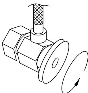
5. After installation is complete, remove the aerator. Turn on the water supply valves and allow both hot and cold water to run at least one minute each. While water is running, check for leaks, especially at hook-ups to supply lines. Tightening nuts slightly will stop any minor leaks.
