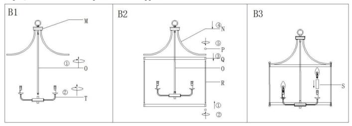
Step B1:Thread the tube (O)onto the bottom of trim(M)
