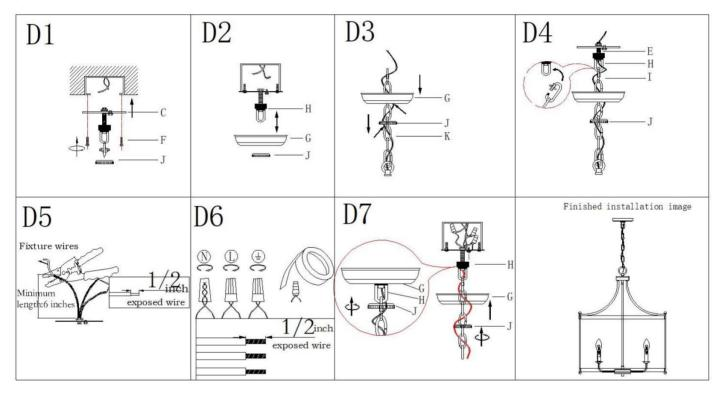
Step D1: Attach the single bar (C) to outlet box with mounting screws (F). The side of single bar marked "GND" must face out
