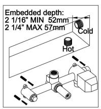
1. Open holes [size of opening is (10.43"-10.71")x(3.62"-3.78")x (2.05"-2.24")inch (LxWxD)] and embedded water pipes (hot and cold inlet pipes, outlet pipes) as required; Install the main body in the embedded hole and connect the pipe.
