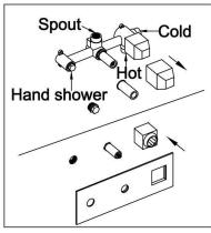
2. Fill the embedded hole after no water leakage, and press the panel to the wall after removing the protective cover.
