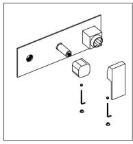
3. Use the hexagon key to install the switch handle and water separator handle and install the color button.
