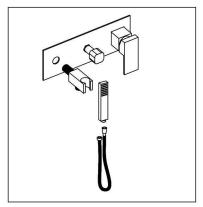
4. Screw the shower seat to the main body mounting hole (be careful to keep it horizontal); use a hose to twist the shower seat interface and the hand-held shower interface together.
