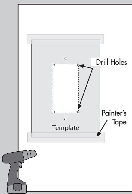
1. Tape the provided wall control template with painter's tape at the desired installation area.
