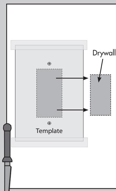
1. Using a drywall punch saw, cut out the interior shape of the template using one of the four drilled corners as a starting point.
