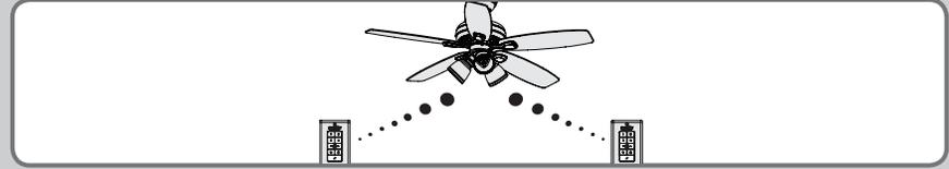
To have multiple remote controls operate one fan, you must pair each additional transmitter to the receiver in the fan. The transmitter that shipped with your fan is already paired.
