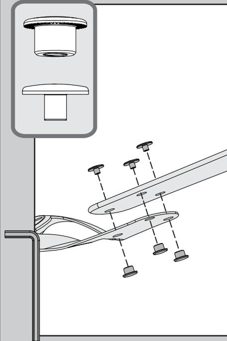
Using the provided Allen wrench, attach each blade to the blade iron assembly using three barrel nuts, found in the ■ hardware bag, and three decorative screws, found in the ▲ hardware bag.
