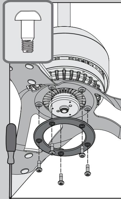
⊗ Align the five holes in the blade iron assembly and the decorative ring with the five holes in the bottom of the motor and partially install the five blade iron screws, found in the ⊗ hardware bag. Once all five screws are partially installed, tighten them securely.
