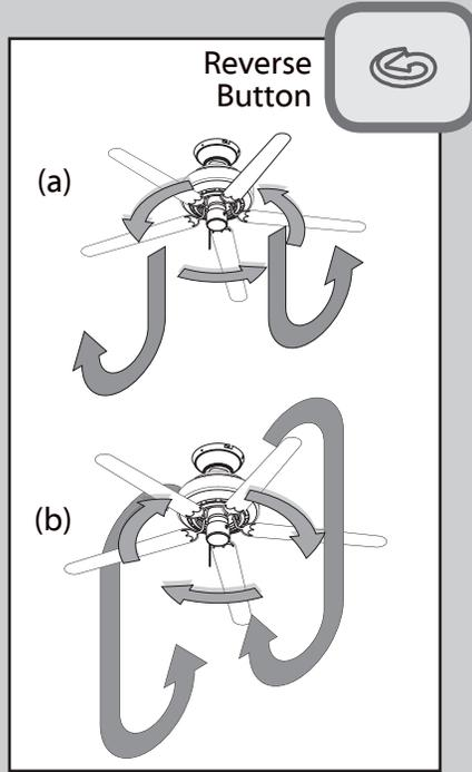
The reverse button on the wall control changes the air flow direction. **In warm weather**, use (a) downward air flow pattern. **In cold weather**, use (b) upward air flow pattern.
