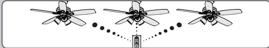
To have multiple fans operated by a single remote control, you must pair the transmitter to each additional receiver. The receiver that shipped with your fan is already paired to the transmitter.
