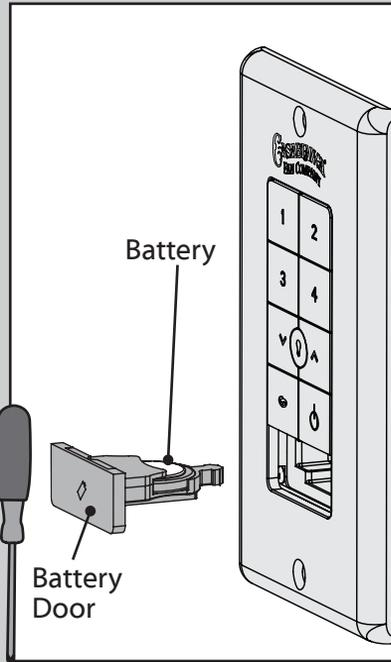
⊗ To change the battery, push on the battery door to eject it. Remove the battery using a small Phillip's head screwdriver. Replace with same type battery, making sure the (+) side is facing down. Replace battery holder and battery door.
