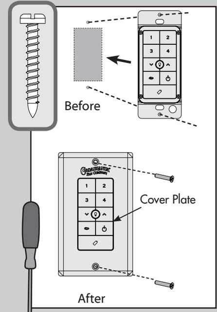
1. Insert the wall control into the dry wall cut out.
