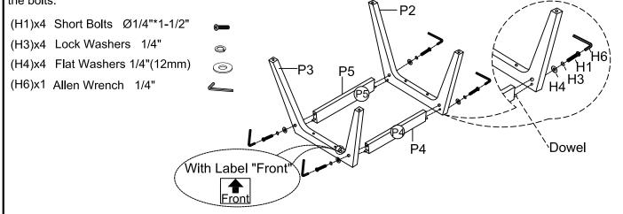
Step 2. Attach the assembled base to the bottom of the chair top (P1). Securely tighten all bolts by Allen wrench (H6), but do not over tighten the bolts.
