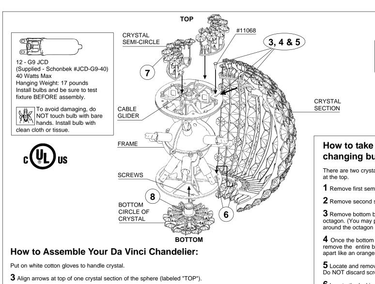
**4** Slide guide tab into slot to line up holes for locking pin.
