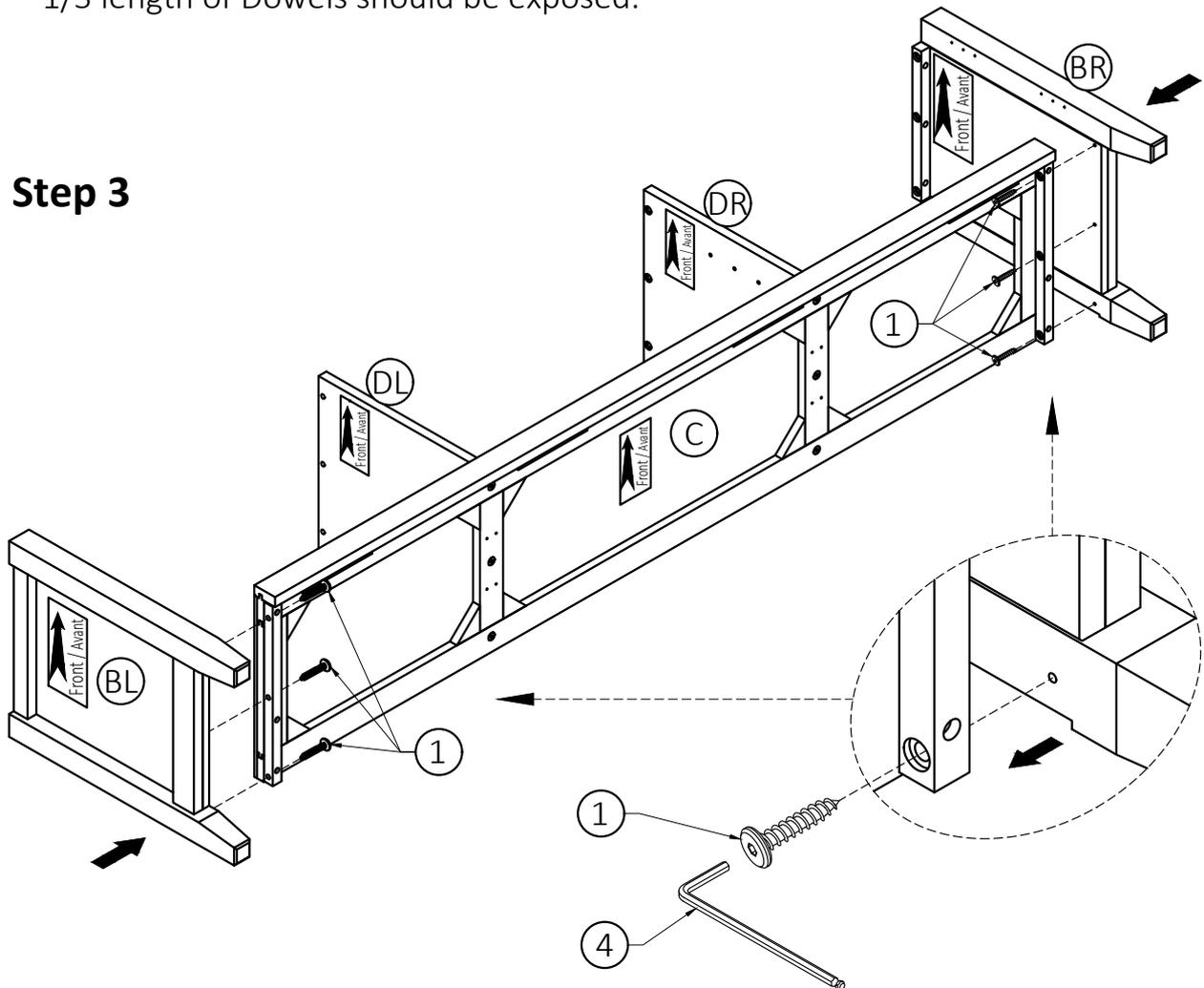
1. Use three Allen Key Screws (1) to attach each Side (BL), (BR) through guide holes from Bottom Shelf (C) to pre-drilled holes of Sides (BL), (BR).
