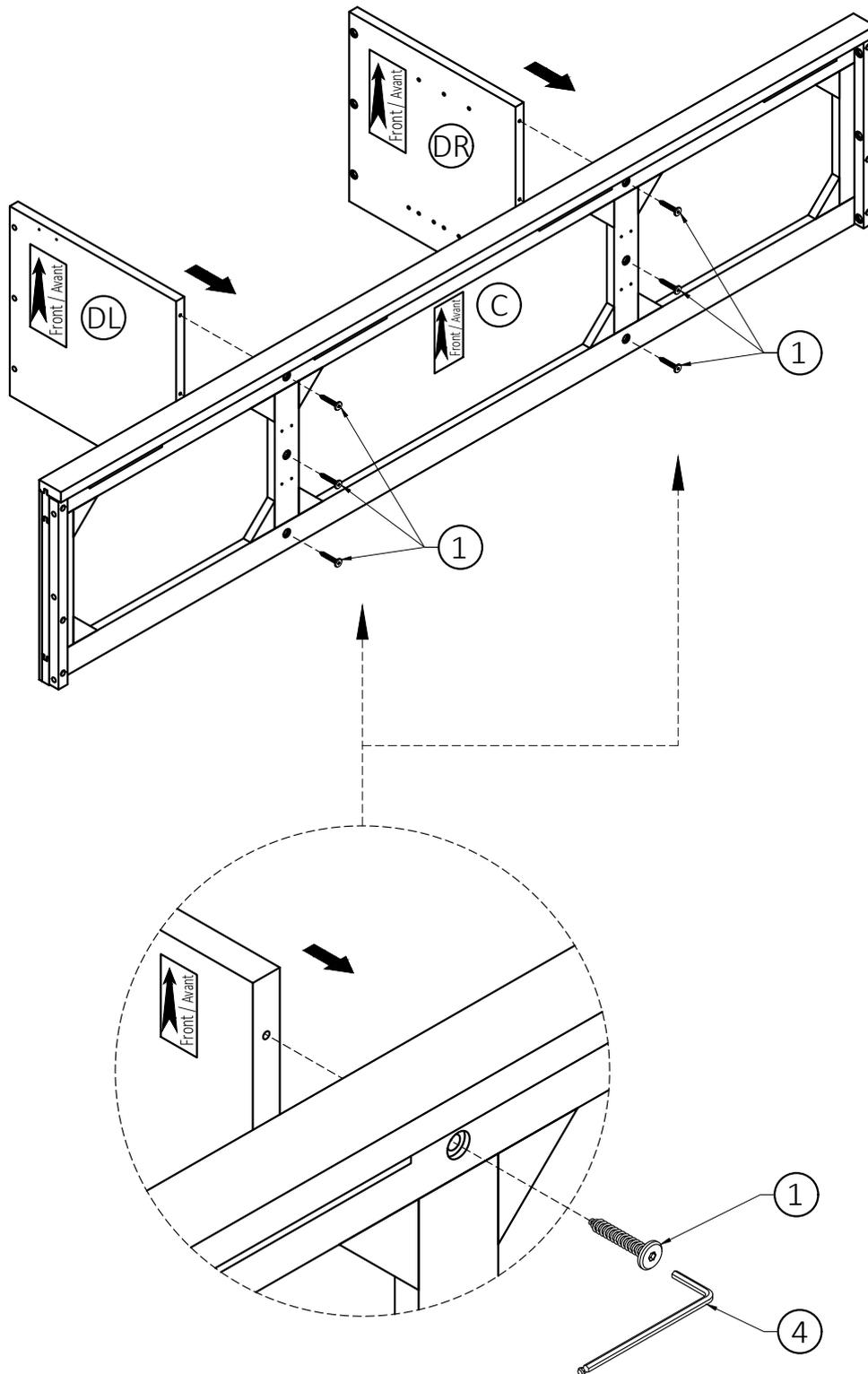
1. Use three Allen Key Screws ① to attach each Divider ①DL, ①DR through guide holes from Bottom Shelf ①C to pre-drilled holes of Dividers ①DL, ①DR.
