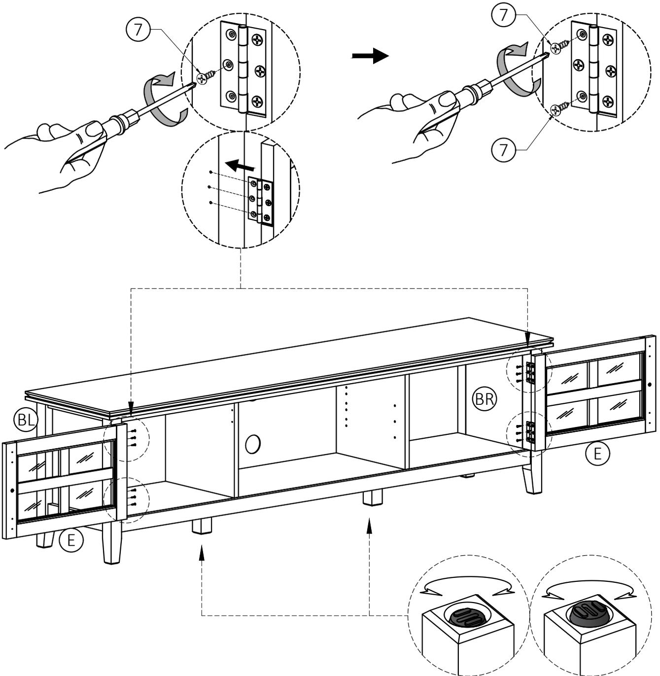
1. Attach hinges on Doors (E) to Sides (BL), (BR) using Phillips Screws (7) into pre-drill holes:
