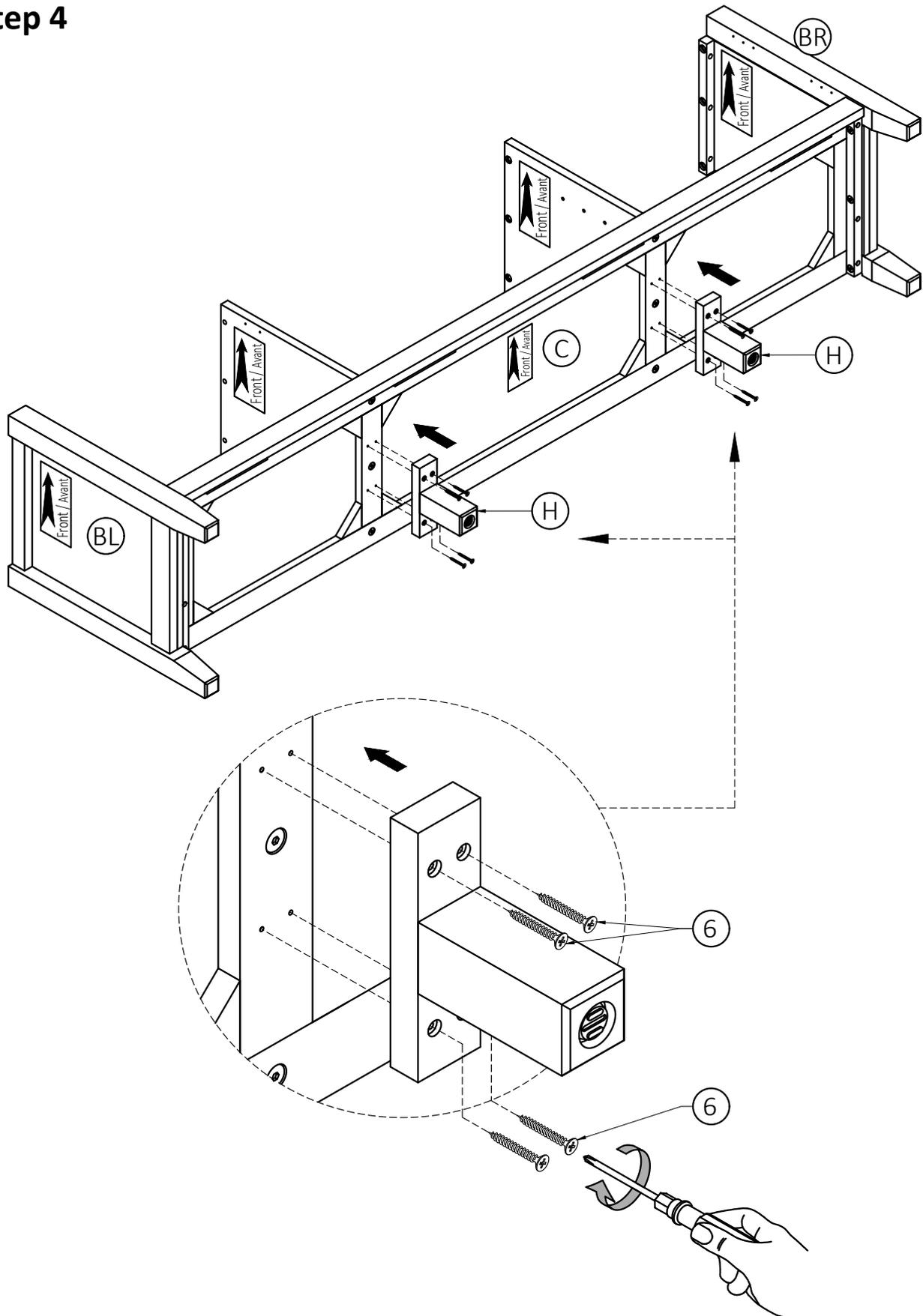
1. Align Bottom Support Legs (H) with pre-drilled holes on back of Bottom Shelf (C). Use Phillips Screwdriver to tighten eight Phillips Screws (6).
