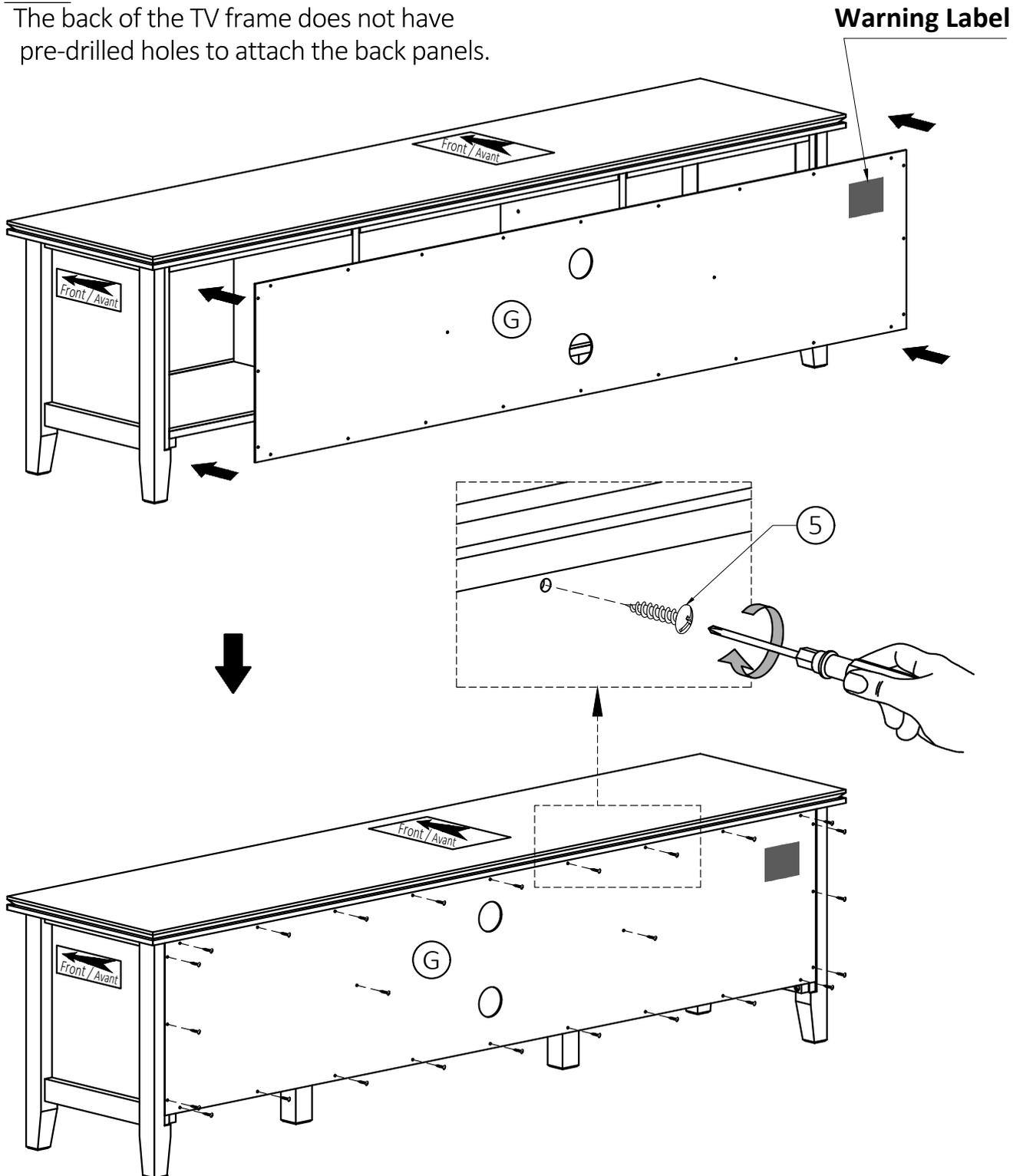
1. Attach the Back Panel (G) to back frame using Phillips Screws Round Head (5) through guide holes from Back Panels.
