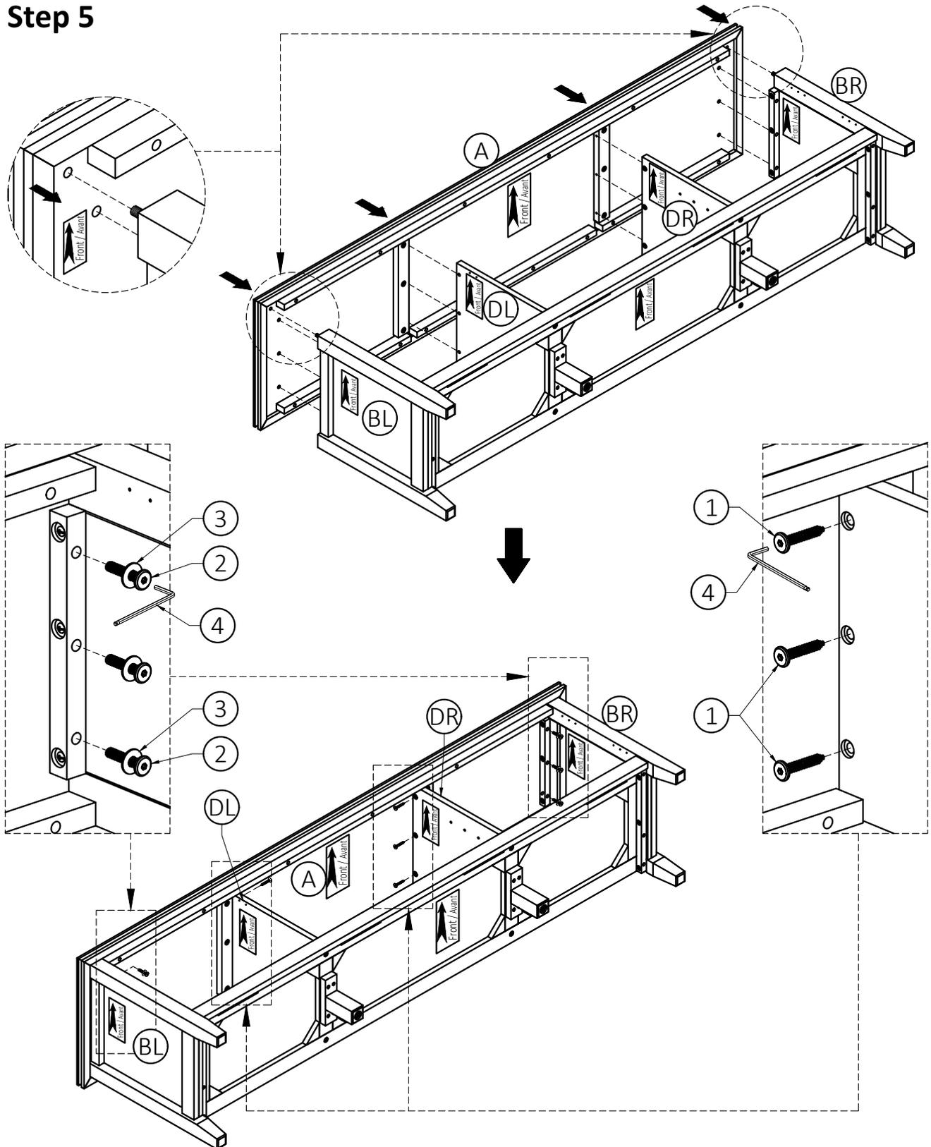
1. Align Wood Dowels with guide holes and attach Sides (BL, BR) and Dividers (DL, DR) to Top (A).
