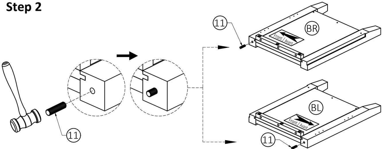
1. Insert one Dowel (11) into guide holes on each Side (BL), (BR).
