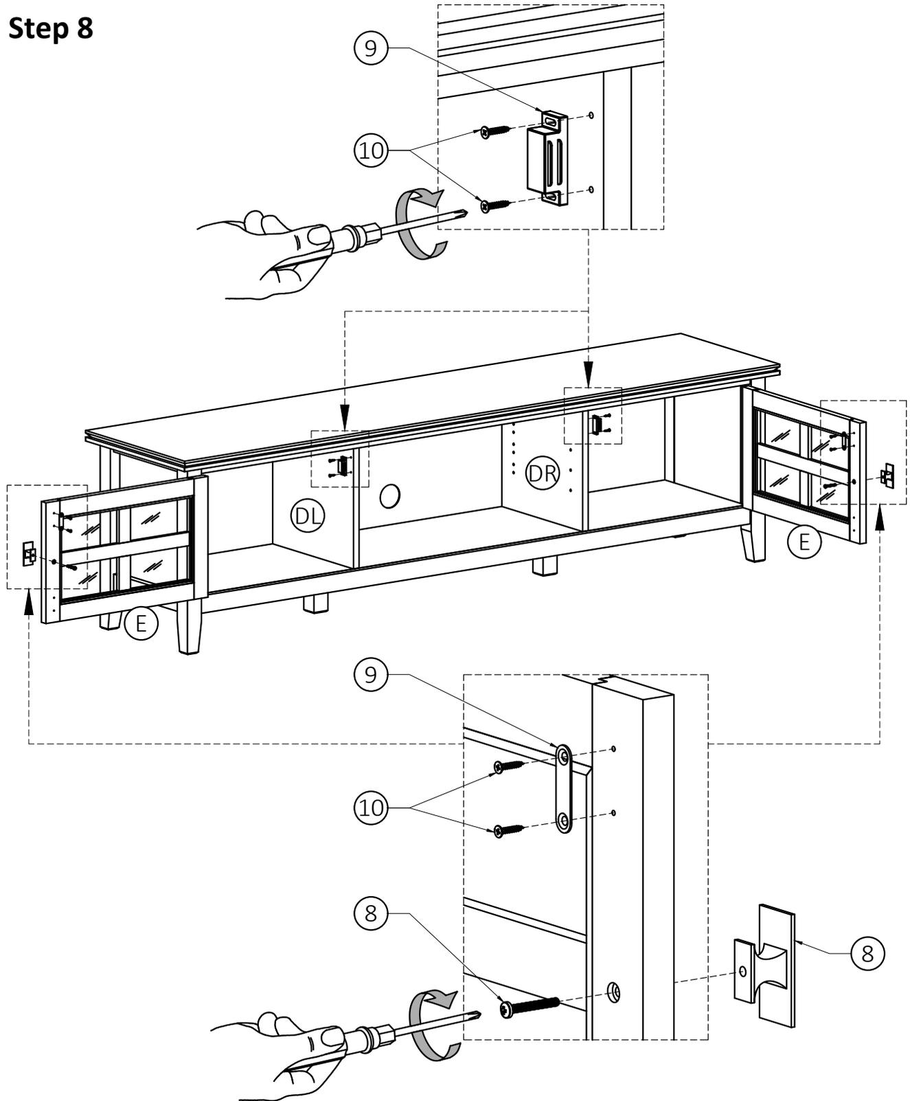
1. Attach Magnet Plates (9) to top corner of Doors (E) using Phillips Screws (10) into pre-drilled holes on Doors (E).
