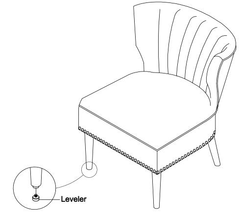
Note: Front legs can be adjusted with adjustable levelers.
