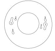
6 For keyholes: Pre-install screws into J-Box and align keyhole slots to screws. Press fixture into box. For all others press fixture into box, then install screws.
