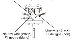
Connect the GROUND WIRE from junction box to GROUND (or GREEN) wire from fixture with a wire nut. Connect the NEUTRAL WIRE from junction box to NEUTRAL (WHITE) wire from fixture with a wire nut. Connect the LINE WIRE from junction box to LINE (BLACK) wire from fixture with a wire nut.
