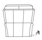
2. Connect the connector from motor to the power cord and transformer
