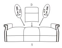
1. Place Bracket into Sleeve and press top of back down firmly to lock your KD back in place
