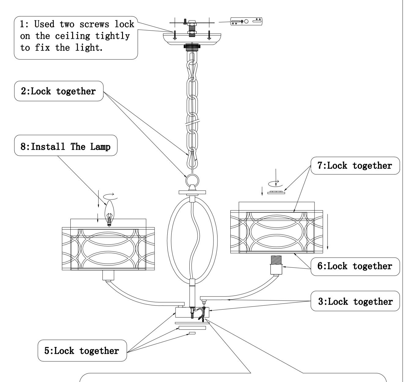
4:Connect all white wires (-) from the arm together, and connect all black wires (+) from the arm together. Do not mix the black and white wires. There are two same main wires, they are thicker than the black and white wires. Connect black wires of the arms together with one of the main wire. Connect white wires of the arms together with the other main wire. The wires connection is finished.
