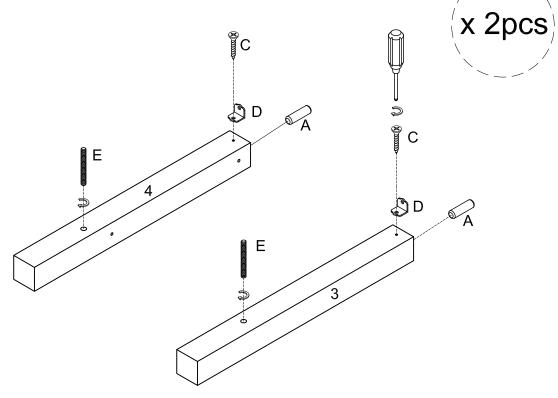
Insert wooden dowel (A) and bolt (E) into part (3,4). Attach bracket (D) to part (3,4) using screw (C) with screwdriver. Repeat this step.
