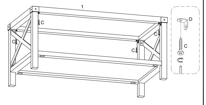
Secure part (1) using screw (C) with screwdriver through bracket (D).
