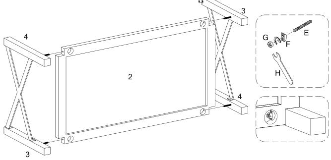
Attach part (3,4) to part (2) using nut (G), washer (F), and bolt (E) with wrench (H).
