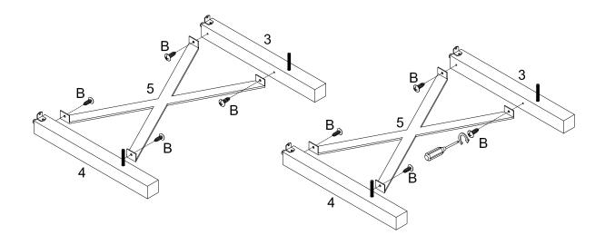
Attach part (3,4) to part (5) using screw (B) with screwdriver.
