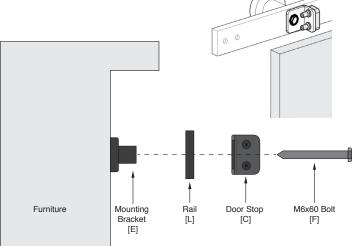
Install the rail, mounting brackets [E], and door stops [C].
