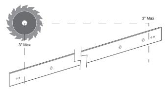
The rail can be trimmed if necessary using a band saw or hacksaw. Use blades suitable for iron or stainless steel depending on your rail.
