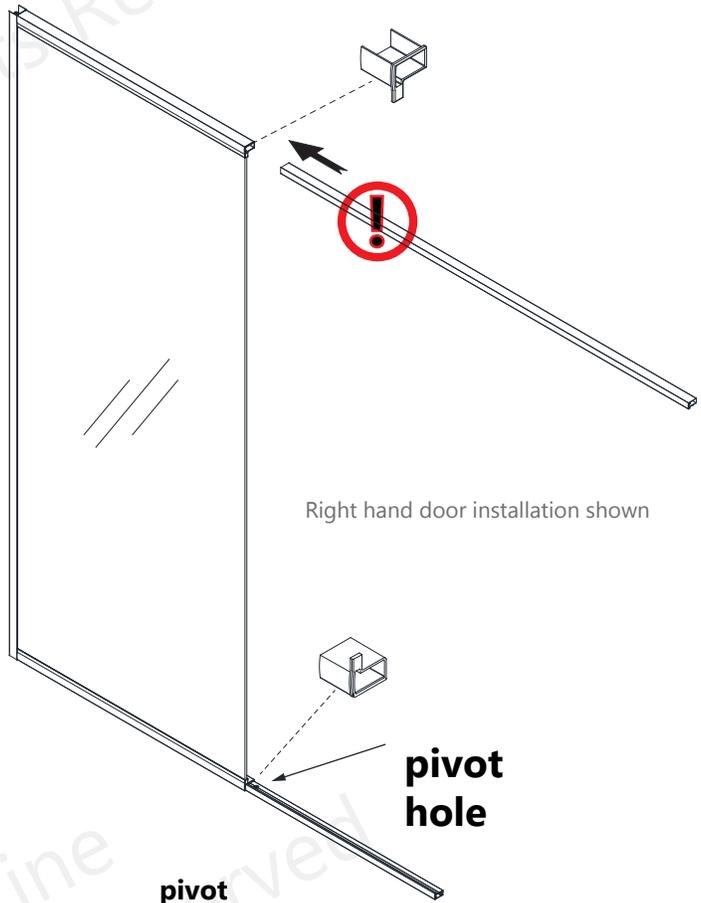
**!** Insert the correct end of the pivot rail based on the model size. (See below)
