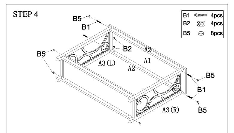
Assemble Side Panels A3(L&R) to Aprons (A2) using Bolts (B1) and Nuts (B2). Then insert Wood Caps (B5) as shown above.
