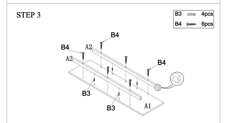
Assemble Aprons (A2) to Top Panel (A1) using Wood Dowels (B3) and Screws (B4).
