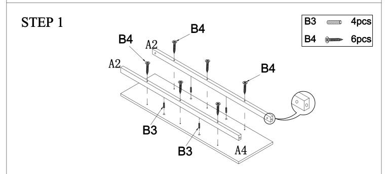
Assemble Aprons (A2) to Bottom Panel (A4) using Wood Dowels (B3) and Screws (B4).
