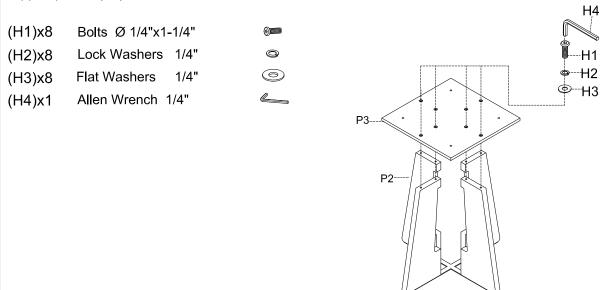
Step 3. Attach the assembled mounting plate (P3) to the bottom of table top (P1) as shown below
