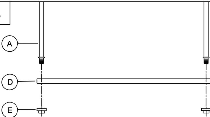
4. Attach flat tube ring (D) to fixture (A), using finial (E) to secure tightly.
