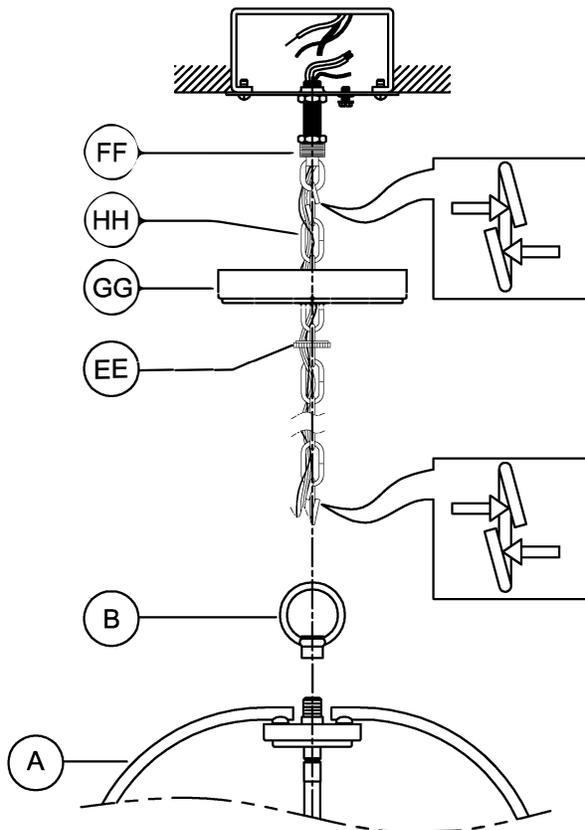
5. Pass the wires through the chain loop (B) and secure tightly onto fixture (A). Weave wires through chain (HH). Pass wires through screw collar (EE) and canopy (GG). Open two links of chain and attach one end to chain loop (B) and the other end to the chain holder (FF). Close the chain links. Pass the wires through the threaded nipple/crossbar.
