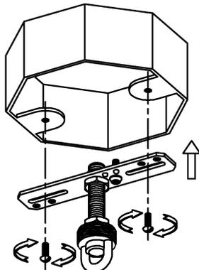
2. Attach assembled parts from step 1 onto outlet box using the mounting screws supplied with the outlet box (not included).
