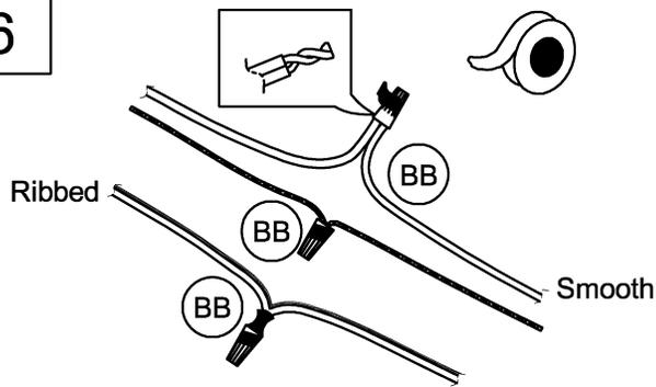
6. Strip 3/8" of insulation from the electrical wire ends. Using wire nuts (BB), connect RIBBED fixture wire to the WHITE supply wire from the outlet box; connect the SMOOTH fixture wire to the BLACK supply wire.
