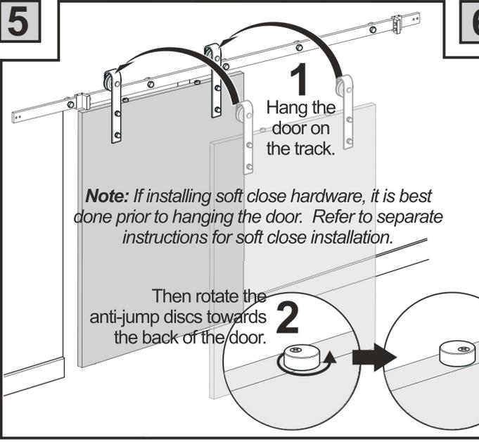
*Note: If installing soft close hardware, it is best done prior to hanging the door. Refer to separate instructions for soft close installation.*
