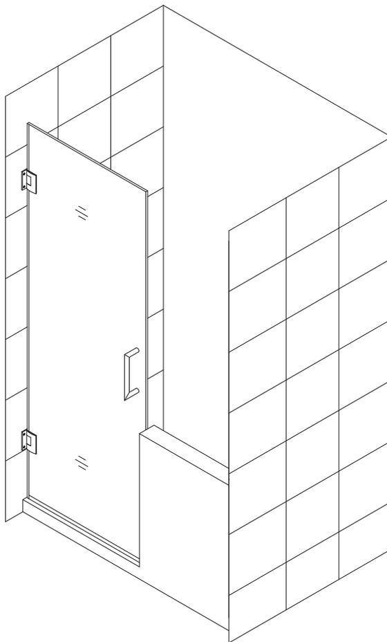
**NOTE:** The Unidoor hinge is factory set to overclose 8°. The following procedure is recommended to ensure proper alignment of the panel glass and door glass.
