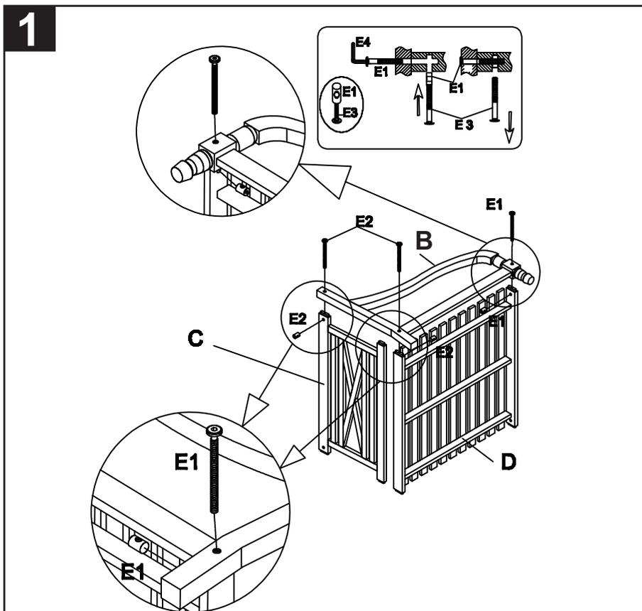
Step1: attach the right side (B) and the back(C) to the seat (D) as shown on the picture by using the Allen bolt (E1) and (E2). Tighten with the Allen key (E4).
