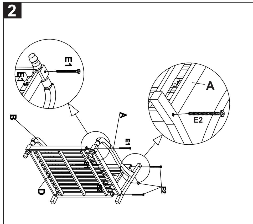
Step 2: put the left side (A) to the chair by using the Allen bolts (E1) and (E2) as shown on the picture. Tighten all with the Allen key (E4).
