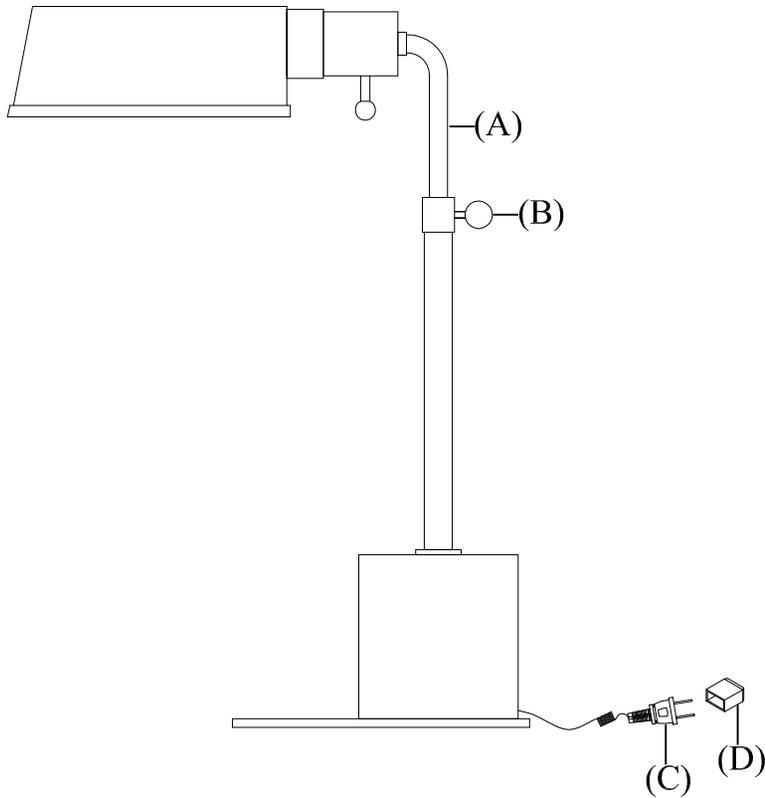
1. Loosen the adjustment key (B) found on lamp stem.
