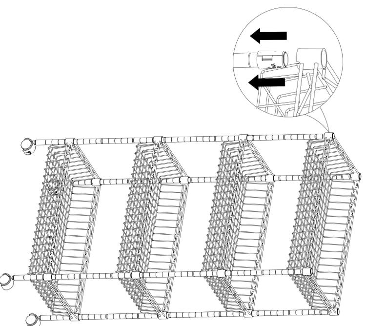
**6** Once all four wire baskets have been installed, pushing firmly down on every basket at corners by rubber mallet to ensure the basket in a place over the plastic clips.
