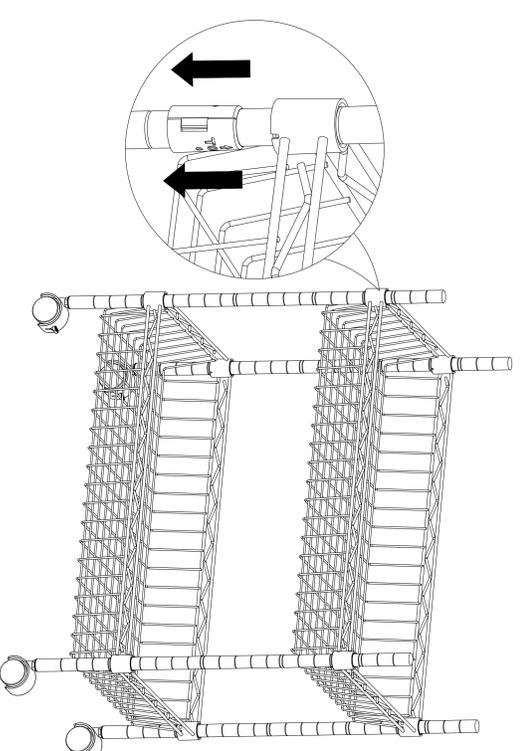
**4** Screw Upper Poles (C) into Lower poles by screw connectors which is already on the upper poles.
