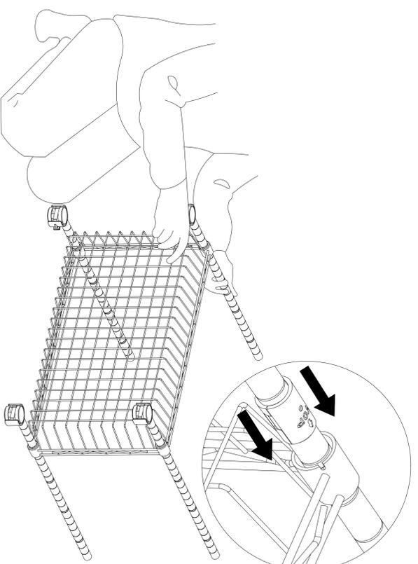
**3** Snap plastic clips into the pole grooves of the lower poles at your desired basket height position. Slide down the basket from top down onto the plastic clips.
