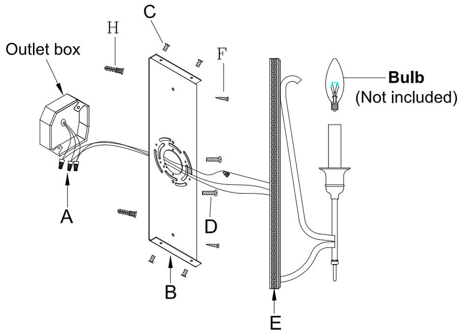
1. Carefully remove the mounting plate (B) from the back plate (E) by removing side screws(C).
