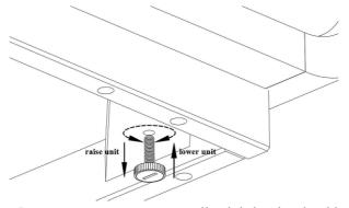
Repeat proses as necessary until unit is level and stable.
