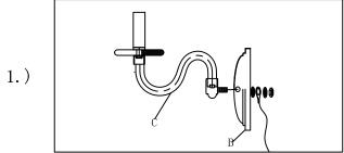
Step.1: Remove mounting bracket (A) from back plate (C) and install to electrical box.
