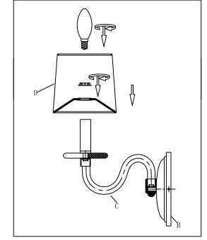
Step.3: Place shade (D) on candle cover and secure using screw ring provided. Then, install 40 Watt candelabra base bulb.
