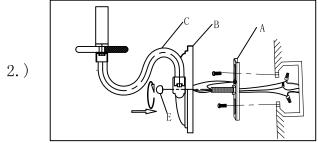
Step.2: Install fixture to mounting backet (A) using finial (E) provided.
