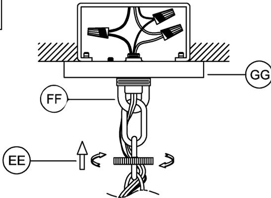
7. Slip the canopy (GG) over the chain holder (FF) Thread the screw collar (EE) onto the chain holder to secure the canopy tightly to the ceiling.
