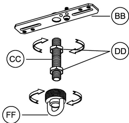
1. Screw threaded nipple (CC) into mounting strap (BB) several turns. Use one hex nut (DD) to secure parts tightly. Thread one hex nut (DD) and chain holder (FF) onto threaded nipple (CC). Tighten the hex nut against the top of the screw collar loop.
