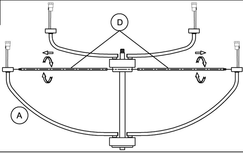
4. Attach tube (D) to fixture (A) and secure tightly.
