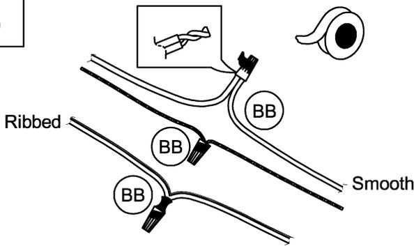
6. Strip 3/8" of insulation from the electrical wire ends. Using wire nuts (BB), connect RIBBED fixture wire to the WHITE supply wire from the outlet box; connect the SMOOTH fixture wire to the BLACK supply wire.
