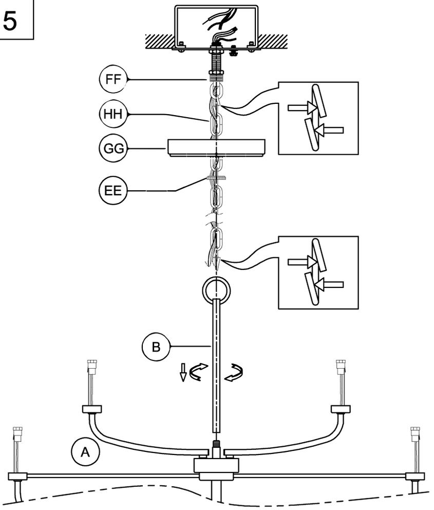
5. Pass the wires through the stem (B) and secure tightly onto fixture (A). Weave wires through chain (HH). Pass wires through screw collar (EE) and canopy (GG). Open two links of chain and attach one end to stem (B) and the other end to the chain holder (FF). Close the chain links. Pass the wires through the chain holder/ threaded nipple/crossbar.
