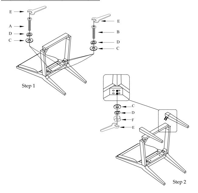
Note: "Before fully tightening the legs, ensure the chair is level"
