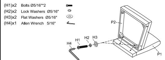
Step 3. Loosely attach the assembled seat frame with cushion (P2) and chair back (P1) to assembled right arm (P4) as shown. Repeat the step to assemble with left arm (P3).
