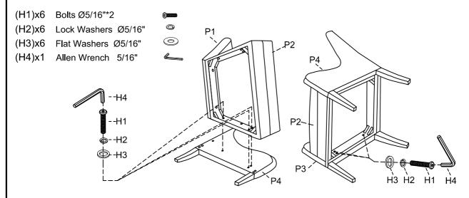
Step 4. Turn the assembled chair to an upright position. Open the back fabric, then attach the back cushion (P1) to the left arm (P3) and right arm (P4) as shown. Make sure the chair is level and securely tighten all bolts with Allen wrench (H4). Cover the back fabric, assembly is complete.
