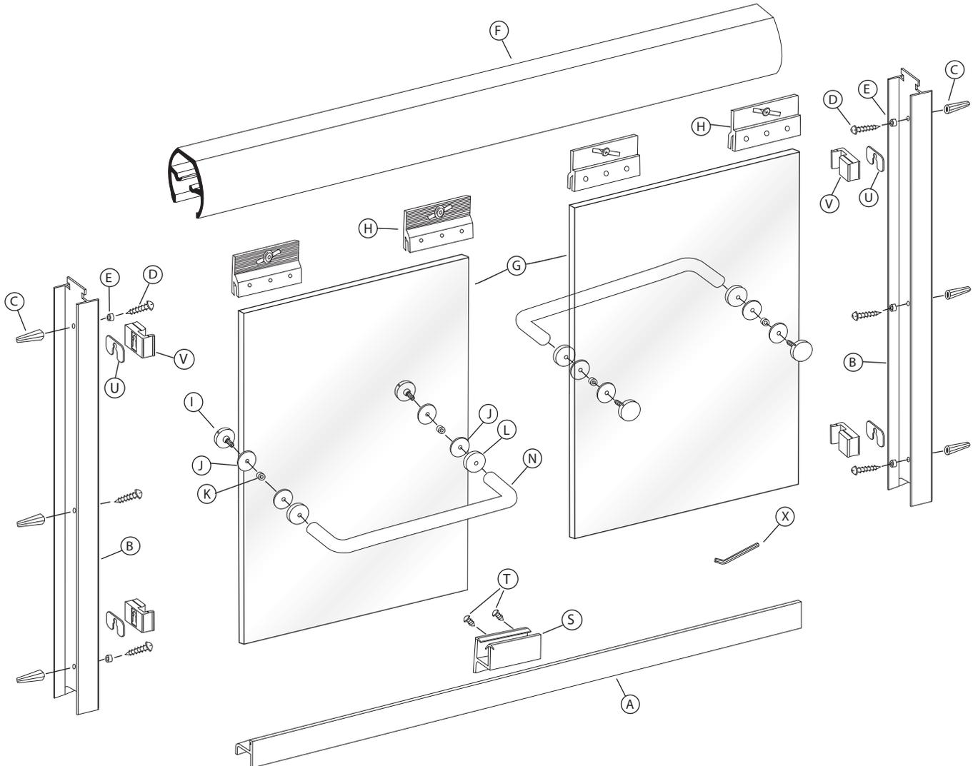
**\*\*If installing on a fiberglass unit you may need to snip outside corner to match corners on wall jamb and tub tracks to match radius on fiberglass unit\*\***
