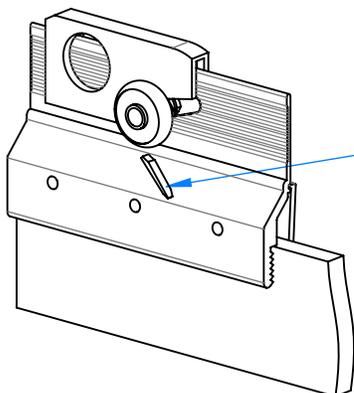
If the Anti-Jump does not stay in the place or if it is difficult to insert, snap off the "roller side leg" leaving one remaining leg.
