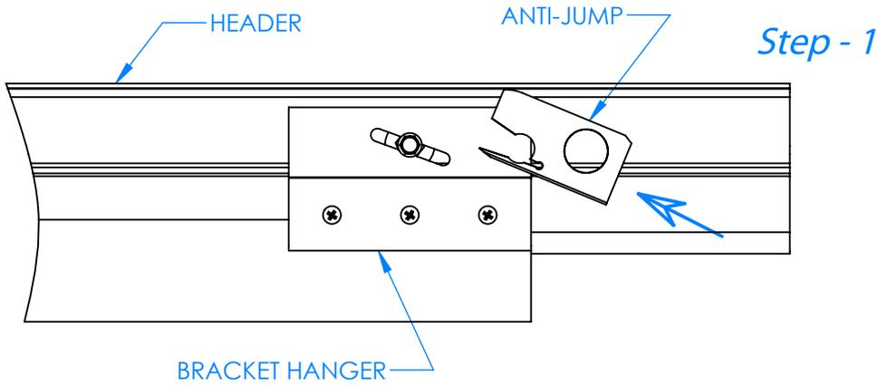
Place one Anti-Jump on each Bracket Hanger: two per panel: four total.
