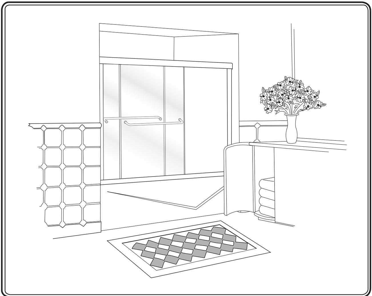
**MAINTENANCE:** Two primary materials are used to manufacture your new shower enclosure: tempered glass and anodized aluminum. To assure a long lasting finish on the enclosure, wipe it down with a towel after each use. Never use a scouring agent to clean the aluminum.
