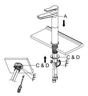
Place the faucet (A) through the mounting hole in the sink until the faucet (A) sits on top of the sink. Secure the faucet (A) to the sink using the rubber (C) and metal washers (D), mounting nut (E) and mounting screws (F) provided.
