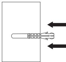
**2c.** Screw a fixing bolt into each anchor using an 8mm spanner until the spanner contacts the wall.
