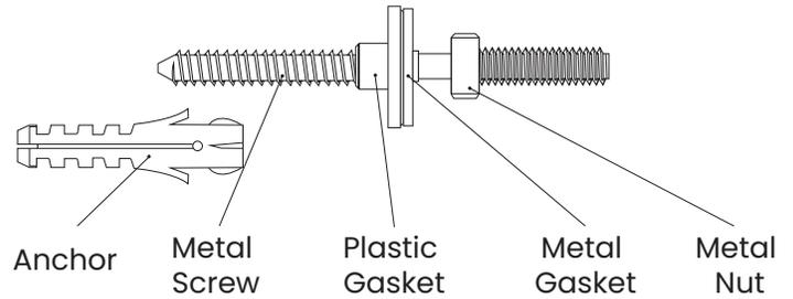
**2a.** Drill two holes in the required position on the wall using a 14mm masonry drill bit, to a depth of 75mm.
