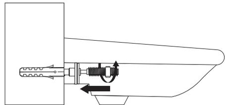
**NOTE:** These fixings are suitable for solid walls only. Plasterboard or stud walls may require specialist fixings (not supplied).
