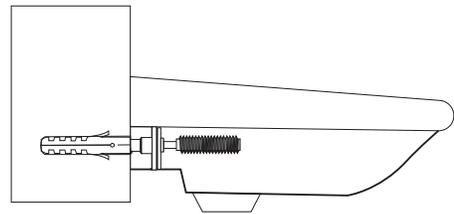
**2e.** Screw a metal nut onto each fixing bolt to secure the basin. Caution: Do not over-tighten, as this may damage the ceramic.
