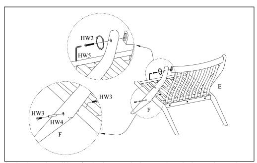
STEP 2: INSERT THE STAINLESS SLEEVE (HW5) INTO THE ARM REST HOLE AND THE SEAT BASE HOLE AND INSERT THE BOLT (HW4) FROM THE INSIDE AND OUTSIDE OF THE LEGS AND SCREW IN THE BOLTS DONT TIGHTEN COMPLETELY INSERT THE BOLTS (HW3) AND SCREW IN THE BOLTS BUT DONT TIGHTEN COMPLETELY
