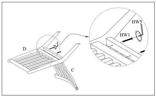
STEP 1: INSERT THE BARREL NUT (HW1) INTO THE HOLE IN SEAT BASE (D). INSERT THE BOLT (HW2) INTO THE HOLE IN BACK REST (C) THEN SCREW IN THE BOLTS DONT TIGHTEN COMPLETELY
