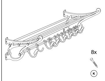
2 Take first iron bar F and insert it from other side starting from one bracket and continue till the other end is visible from the other side of bracket into square pipe through slots in the both sides of brackets. Loosely fasten screw nuts J on the end of bar which is visible from outer side of bracket.
