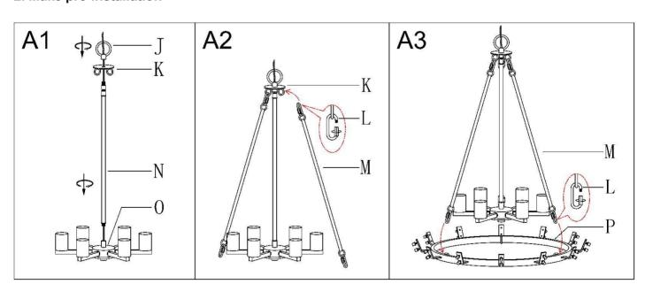
Step A1 » 1) Screw loop (J) onto fixture loop assembly (K).
