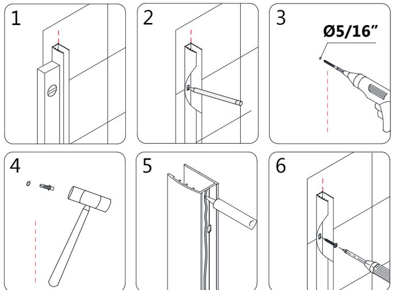
4. Be sure the **Panel Glass (#03)** and **Glass Profiles (#01)** have had time to set up before handling. Insert each assembled **Panel Glass (#03)** and **Glass Profile (#01)** into the installed **Wall Profiles (#03)** and check the panels for plumb. If necessary, adjustments can be made by moving the **Glass Profiles (#01)** within the **Wall Profiles (#03)**. Use caution not to pull the **Panel Glass (#03)** out of the **Glass Profiles (#01)**. (Fig 4a and Fig 4b)
