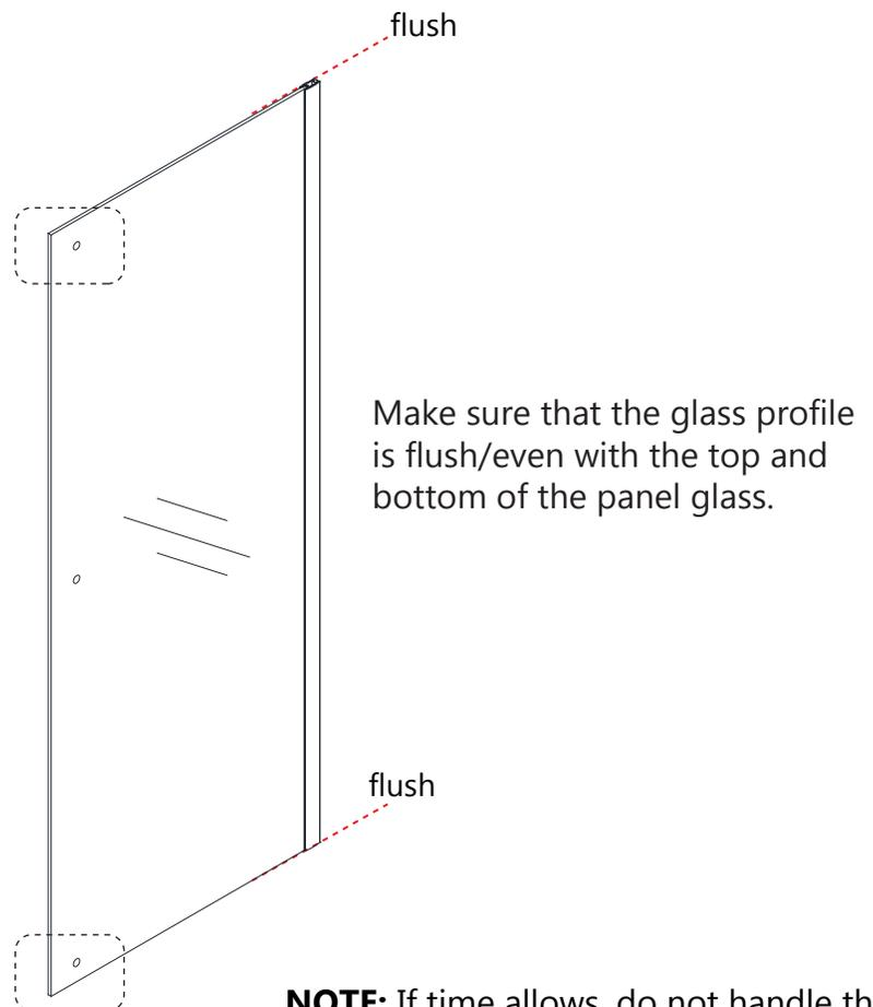
Make sure that the glass profile is flush/even with the top and bottom of the panel glass.
