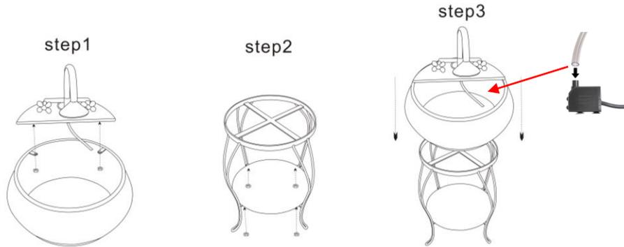
1. Take the fountain sink faucet (C) and place over fountain sink bowl (D). Match the 2 holes from the faucet (C) over the 2 screws on the bowl (D). Once inside, secure by using two (2) nuts (B) and tighten clockwise. See above **Step 1**.
