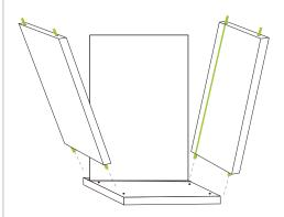
Arrange vertical zBoard with grooves facing backboard as shown.
