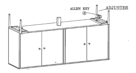
USE THE ALLEN KEY TO SCREW THE ALLEN BOLT.
