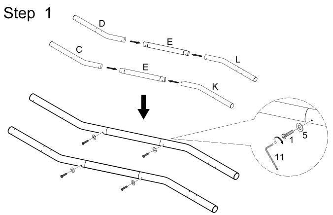
Slide curved post sections (C,K) and curved post sections (D,L) onto post sections (E). Secure the post sections together using medium bolts (1) with small washers (5). Tighten medium bolts (1) with small wrench (11).
