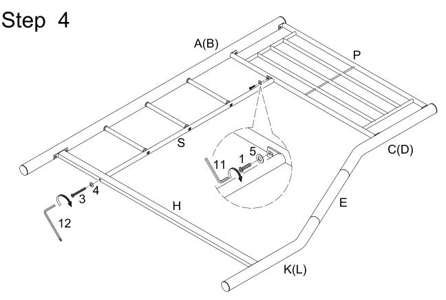
Secure ladder rail (S) to guardrail (P) using medium bolt (1) with small washer (5). Secure ladder rail (S) to crossbar (H) using large bolt (3) with large washer (4). Tighten bolts with wrenches (11,12). Repeat this step on the opposite side of the bunk bed.
