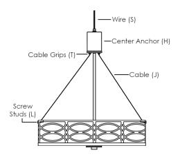
8 Attach Cables (J) to Screw Studs (L). To allow the Diffuser (R) to sit properly onto metal ring on Shade (M), tighten/straighten Cables (J) by pushing Cables (J) into Cable Grips (T) on bottom of Socket Assembly (I).
