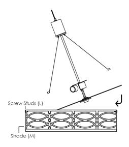
7 Place Shade (M) on a sturdy surface with Screw Stud (L) side up. At an angle, place Diffuser (R), Center Anchor (H) and Socket Assembly (I) onto metal ring on the bottom of Shade (M). Be careful to avoid Screw Studs (L) on the top of Shade (M).
