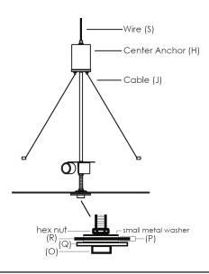
Attach Diffuser (R) shiny side facing away from Socket (K).
