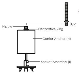
Remove the decorative ring from the top of Center Anchor (H). Slide up Center Anchor (H) exposing the nipple. Adjust hex nut on the nipple 1/2" from bottom. Screw the bottom of the nipple into the top of Socket Assembly (I) until you reach the bottom hex nut. Replace Center Anchor (H) over the nipple and lock in place with the decorative ring.
