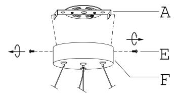
4 » Attach mounting plate (A) to the outlet box with mounting screws (D).
