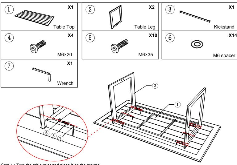
Step 1: Turn the table over and place it on the ground where the exterior finish will not be scratched.
