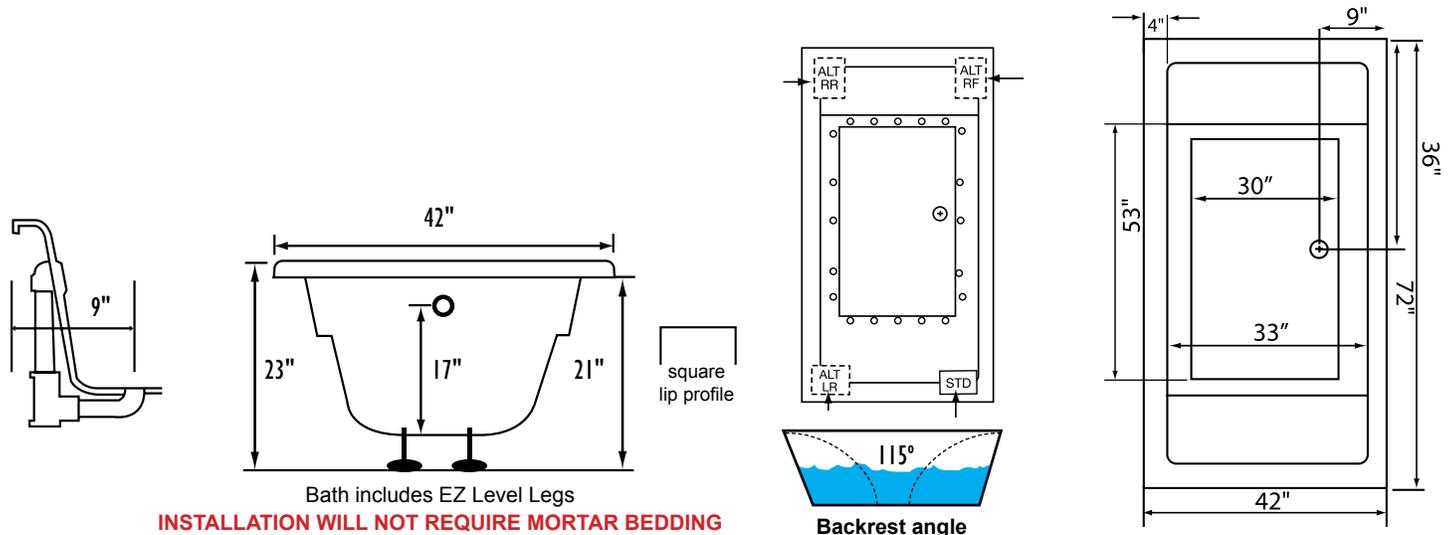
**NOTE:** Graphics may not be to scale. Specifications and features are subject to change without notice and are  $\pm .25"$ . All final measurements should be taken from **tub on site**. Access 18"x 18" or larger is required for each pump. Some pump locations and plumbing may extend beyond the perimeter of the bath.
