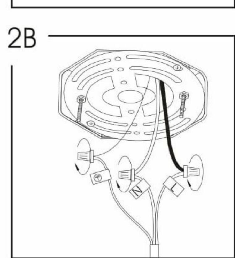
Strip 3/4" of insulation from wire ends. Connect house ground wire to fixture ground wire marked with symbol. Twist wires together using wire nut. Connect black house wire to the fixture wire marked "L". Twist wires together using wire nut. Connect white house wire to the fixture wire marked "N". Twist wires together using wire nut.
